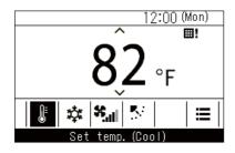
When "#!" is displayed, be sure to clean the filters and then do a reset.
