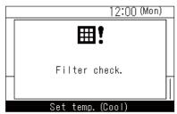
• If the air conditioners are operated while "■!" is displayed, then "Filter check." is displayed. Press an operation button while it is displayed or leave it for at least 5 seconds and the display will disappear.
