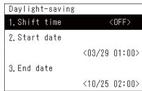
**2** Select "Daylight-saving" using [∧] and [∨], and then press [●] (Confirm).
